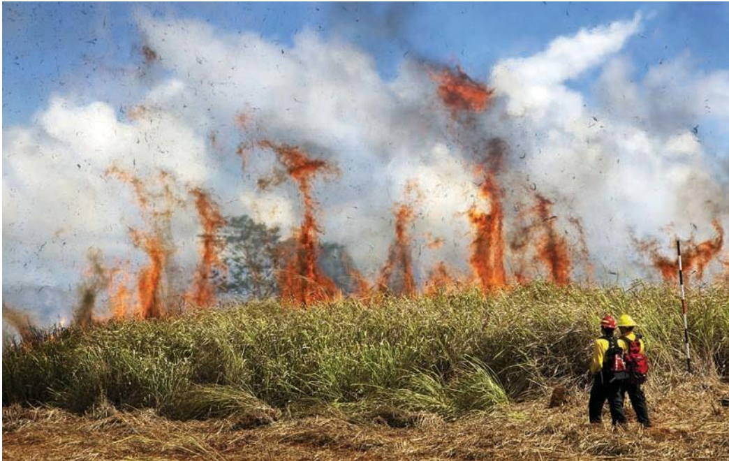
Figure 7.2. An experimental fire in guinea grass illustrating high fire intensity (4–5 meter flame lengths) despite relatively benign fire weather (70 percent relative humidity, 5 mph winds) (photo by Clay Trauernicht, 2013).
